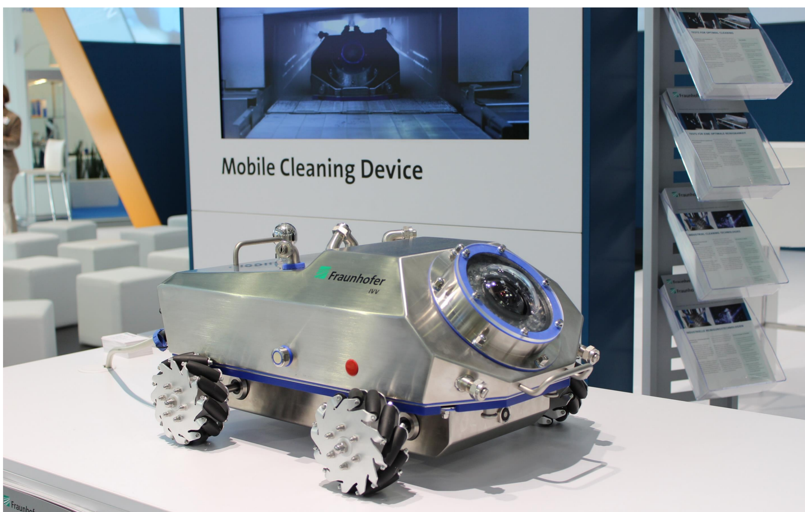
Fig. 2: Self-driving prototype of the MCD
